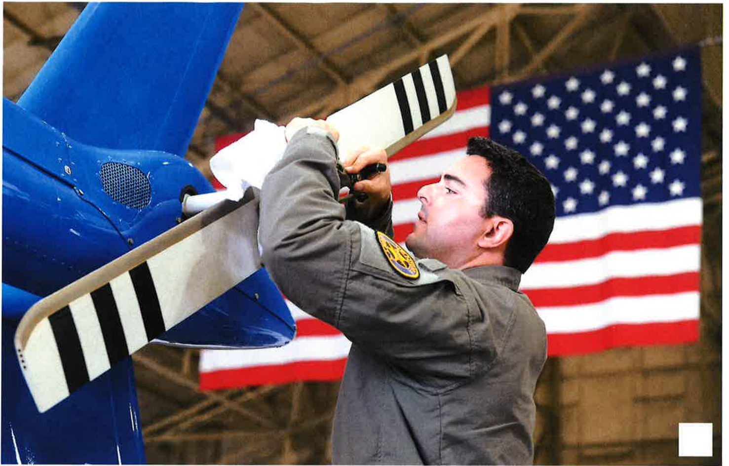
Ventura County Sheriff's pilot Alex Keller inspects the small rotor placed vertically at the tail of Helicopter 3 at the Camarillo Airport.
