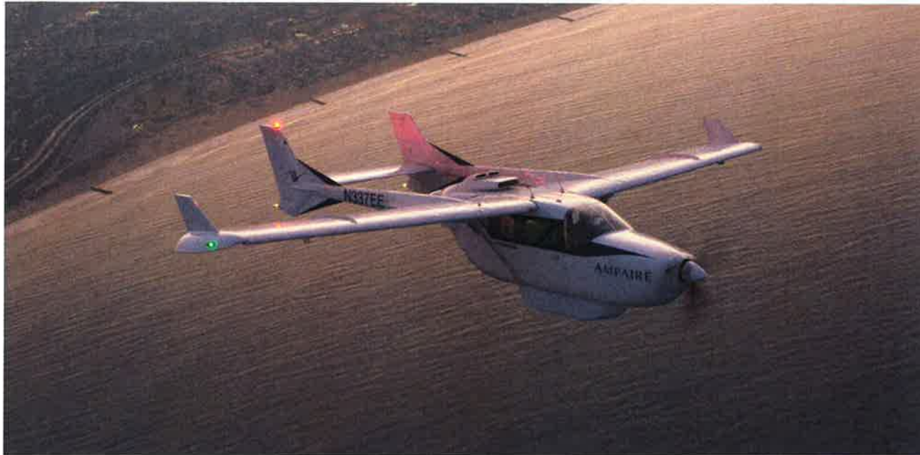
A twin-engine Cessna 337 Skymaster with its engines arranged in a unique push-pull configuration has been retrofitted by Ampaire as its Electric EEL, with an electric motor replacing the forward piston engine. (Photo: Ampaire)
