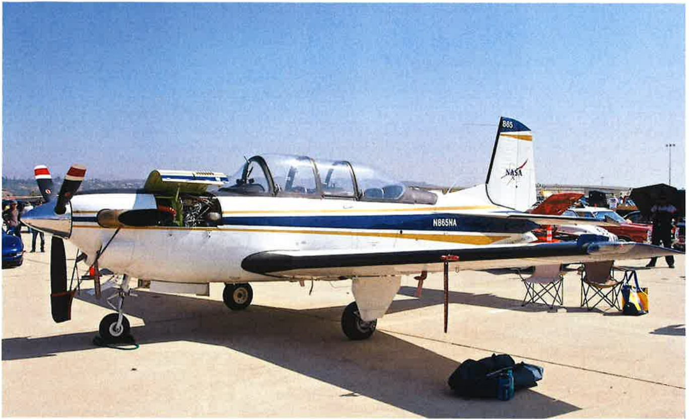
A NASA operated T-34C Mentor, used for pilot proficiency and low-speed chase duties.
