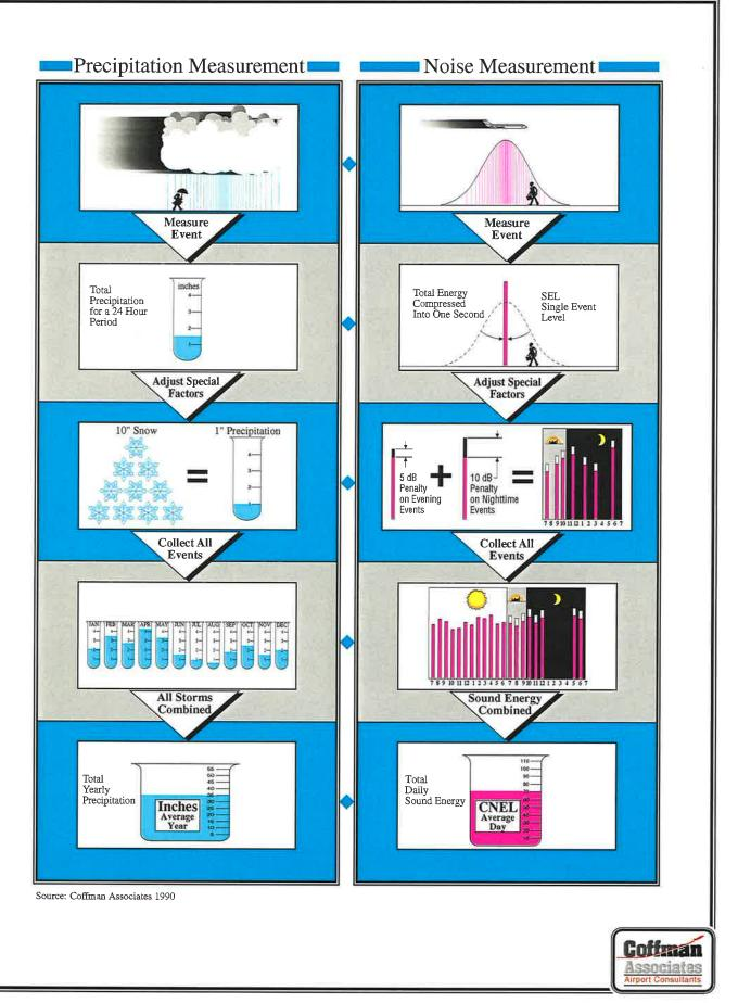
CAL.Sound Exhibit D PRECIPITATION AND NOISE MEASUREMENT COMPARISON
