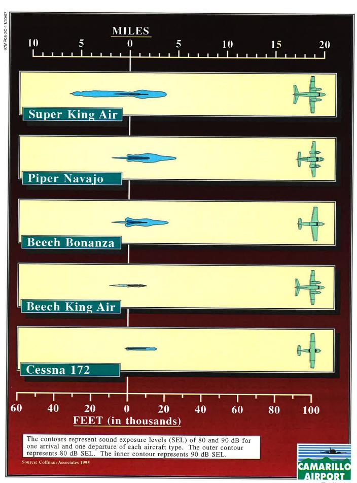
Exhibit 2C PROPELLER AIRCRAFT NOISE FOOTPRINT COMPARISON
